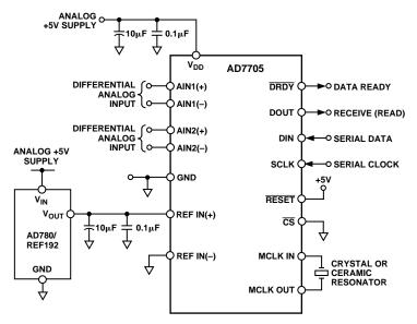
Figure 10. AD7705 Basic Connection Diagram
