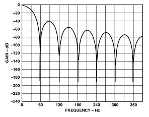
Figure 12. Frequency Response of AD7705 Filter
