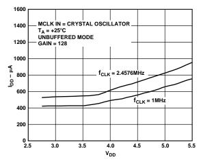
Figure 15. I<sub>DD</sub> vs. Supply Voltage
