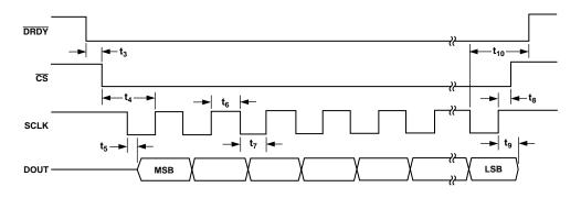
Figure 16. Read Cycle Timing Diagram
