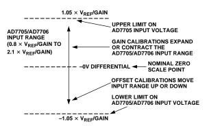
Figure 13. Span and Offset Limits
