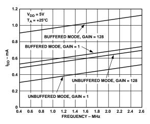
Figure 6. Typical I<sub>DD</sub> vs. MCLKIN Frequency @ 5 V
