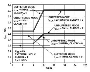
Figure 4. Typical I<sub>DD</sub> vs. Gain and Clock Frequency @ 3 V
