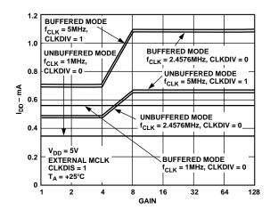
Figure 7. Typical I<sub>DD</sub> vs. Gain and Clock Frequency @ 5 V
