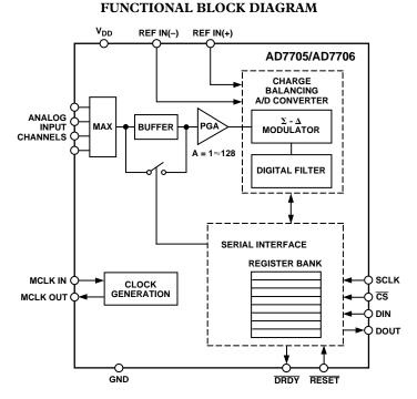
using the input serial port. The part contains self-calibration and system calibration options to eliminate gain and offset errors on the part itself or in the system.
