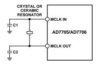
*Figure 14. Crystal/Resonator Connection for the AD7705/AD7706*
