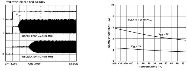
Figure 8. Typical Crystal Oscillator Power-Up Time
