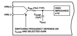
Figure 11. Unbuffered Analog Input Structure
