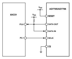
Figure 20. AD7705/AD7706 to 8XC51 Interface
