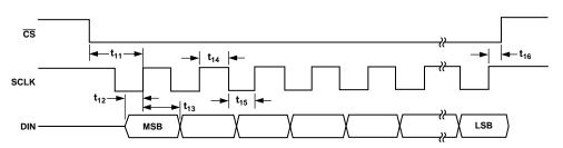
Figure 17. Write Cycle Timing Diagram
