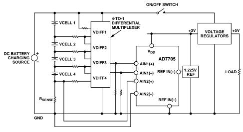
Figure 26. Battery Monitoring Using the AD7705
