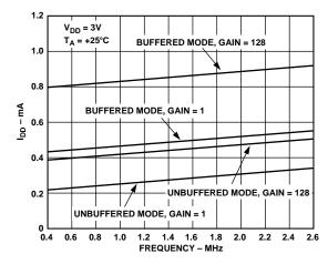
Figure 3. Typical I<sub>DD</sub> vs. MCLKIN Frequency @ 3 V
