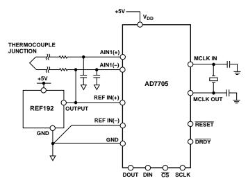
Figure 23. Temperature Measurement Using the AD7705
