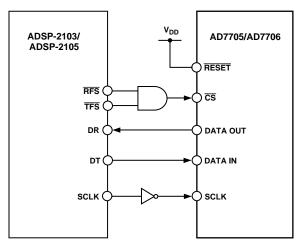
Figure 21. AD7705/AD7706 to ADSP-2103/ADSP-2105 Interface
