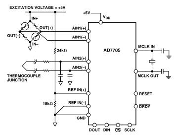
Figure 22. Pressure Measurement Using the AD7705
