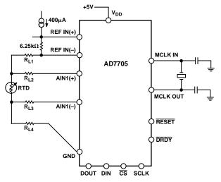
Figure 24. RTD Measurement Using the AD7705
