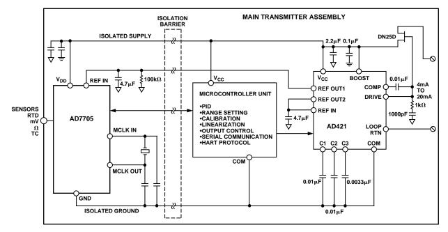
Figure 25. Smart Transmitter Using the AD7705
